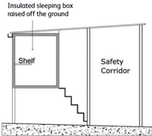
Pre-2013 standard with space under the box taken into the overall footprint allowance
